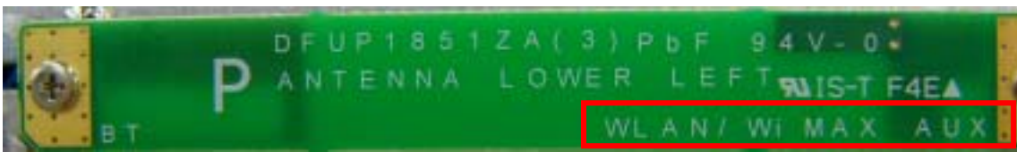
WLAN Aux TX/RX Antenna
