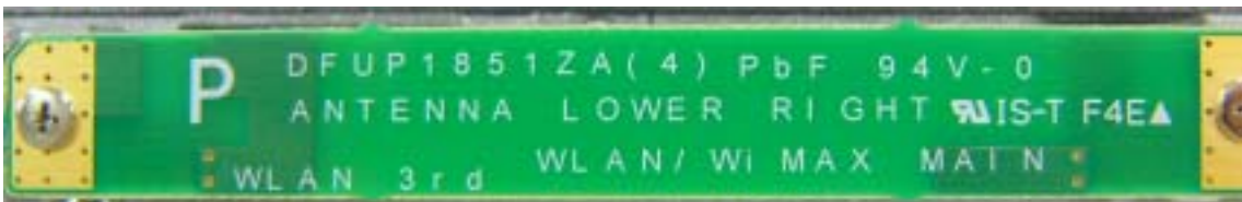
WLAN Main TX/RX Antenna
