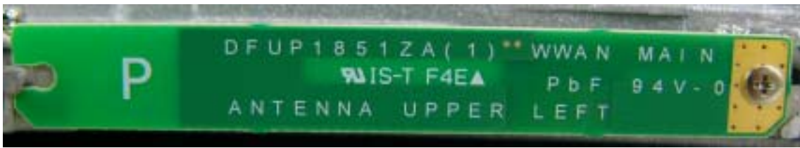
WWAN Main TX/RX Antenna
