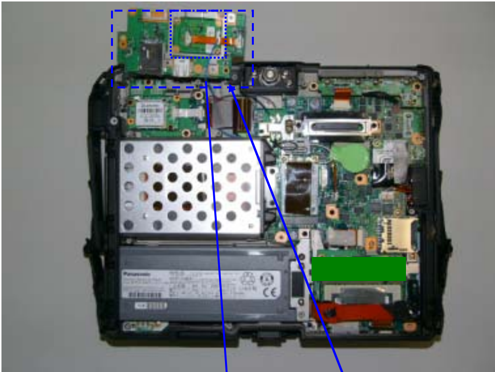
Reverse side of RF PWB
