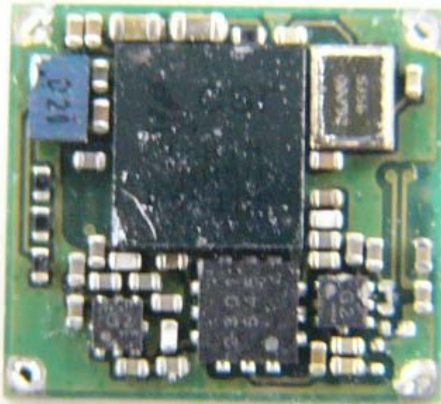
Bluetooth Module inside Top View
