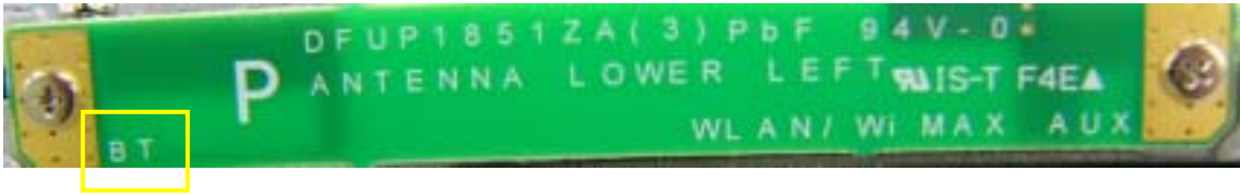
Bluetooth TX/RX Antenna
