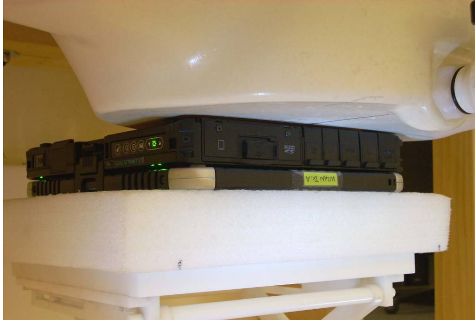
Figure 19-3 SAR Test Setup Photo 3 (Laptop Chain A)
