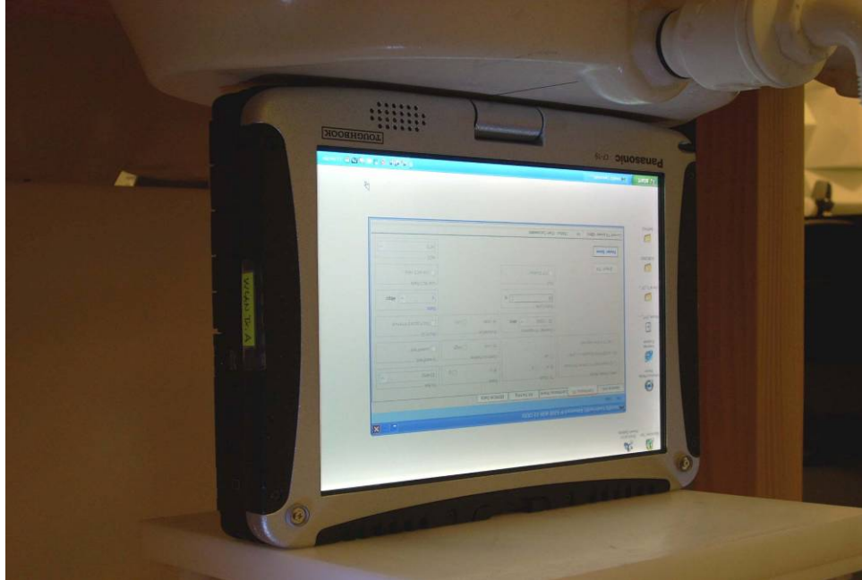
Figure 19-1 SAR Test Setup Photo 1 (Tablet Bottom)
