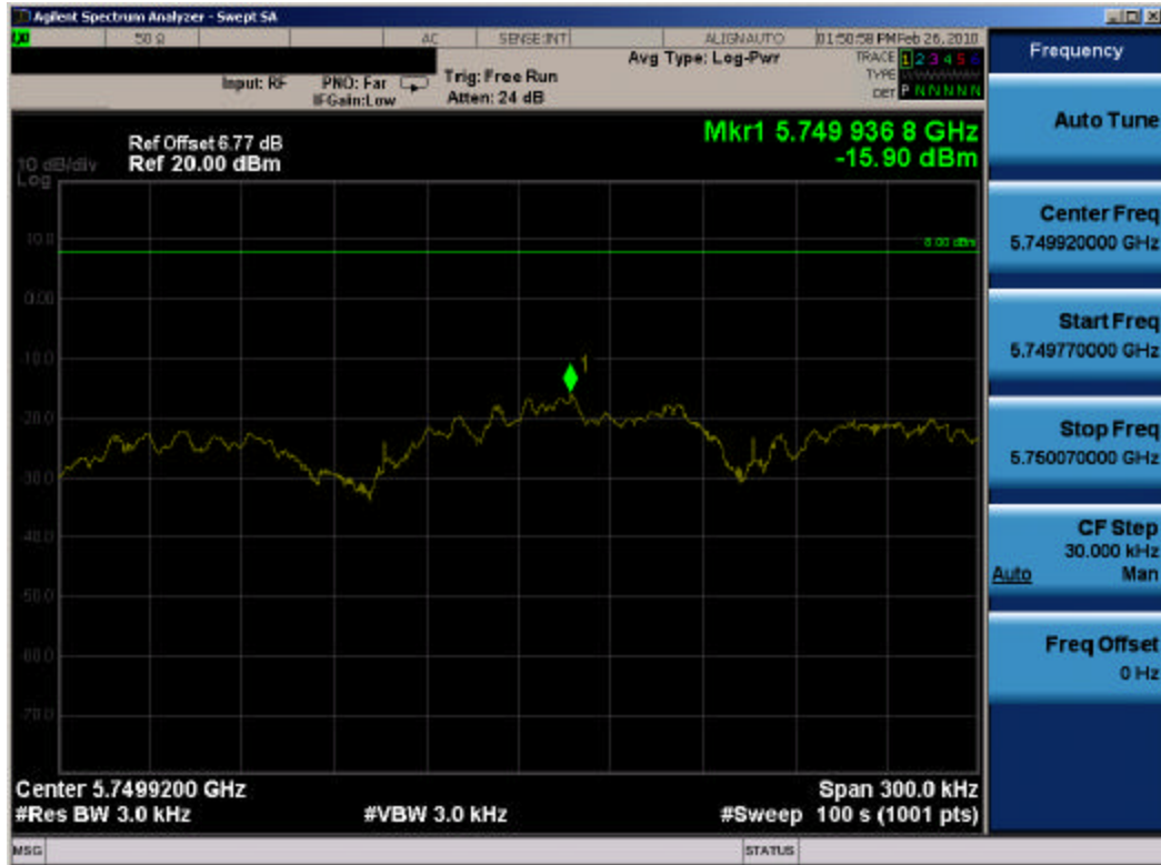
Plot 6-29. Power Spectral Density (802.11n (5.8GHz) Dual Transmit Mode – Ch. 151) – Chain B
