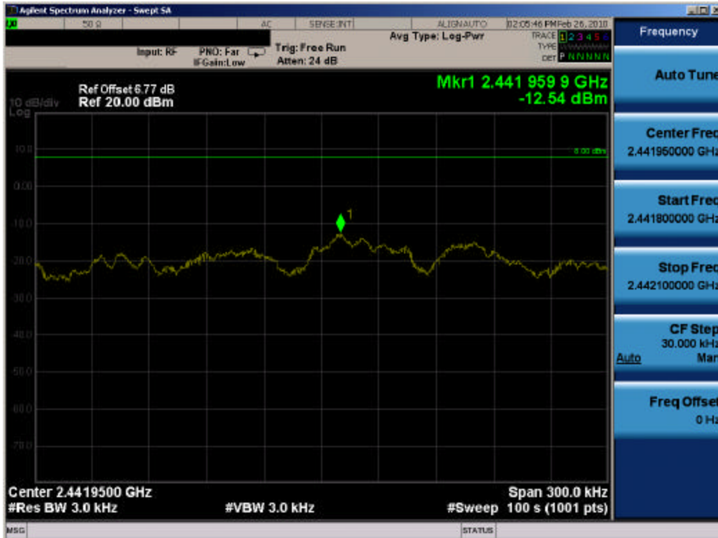
Plot 6-27. Power Spectral Density (802.11n (2.4GHz) Dual Transmit Mode – Ch. 6) – Chain B
