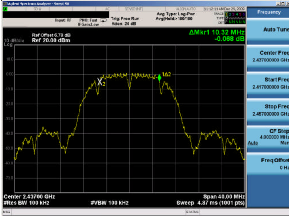
Plot 6-1. 6dB Bandwidth Plot (802.11b – Ch. 6) – Chain A
