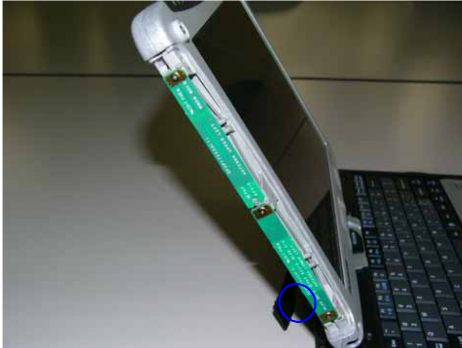
WLAN Main TX/RX Antenna
