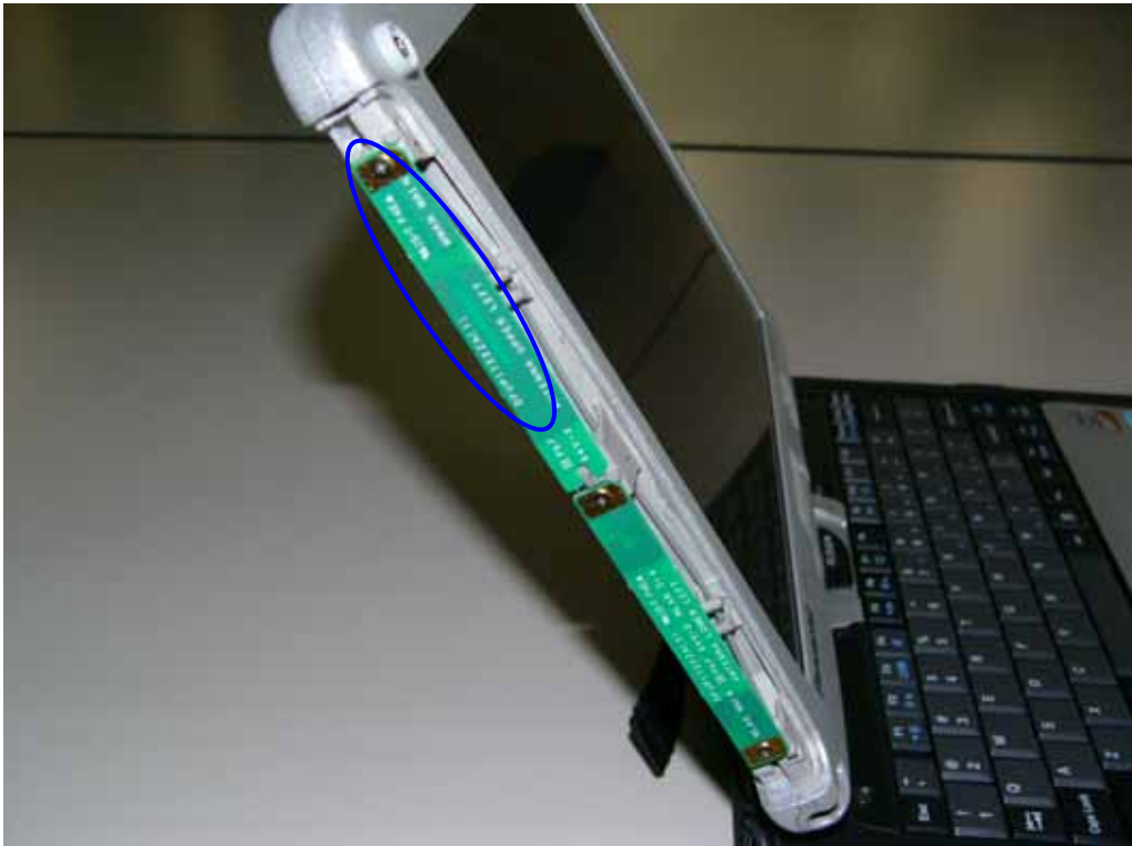
WWAN Main TX/RX Antenna
