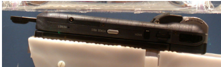
Figure 8-2 CompactFlash radio card in PDA host configuration
