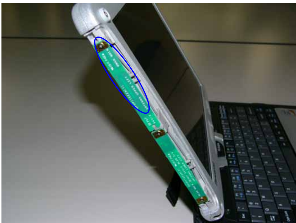
HSDPA Main TX/RX Antenna
