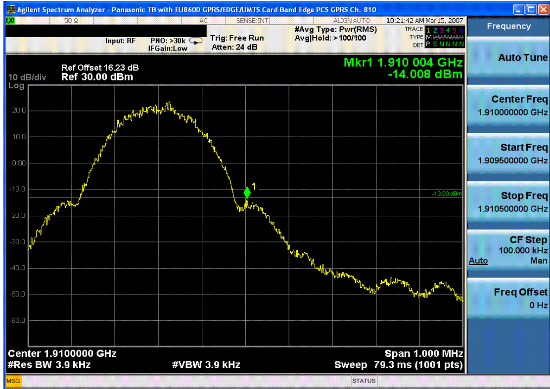
Plot 7-21. Band Edge Plot (PCS GSM Mode – Ch. 810)
