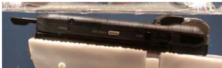
Figure 8-2 CompactFlash radio card in PDA host configuration
