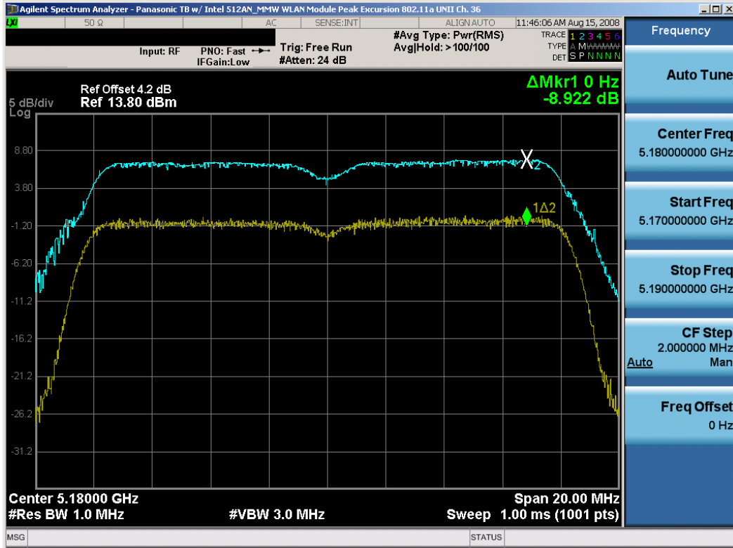
Plot 6-33. Peak Excursion Ratio Plot (802.11a (UNII) – Ch. 36)
