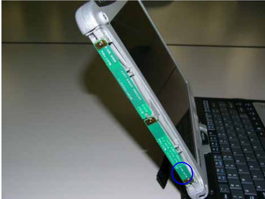
WLAN Main TX/RX Antenna
