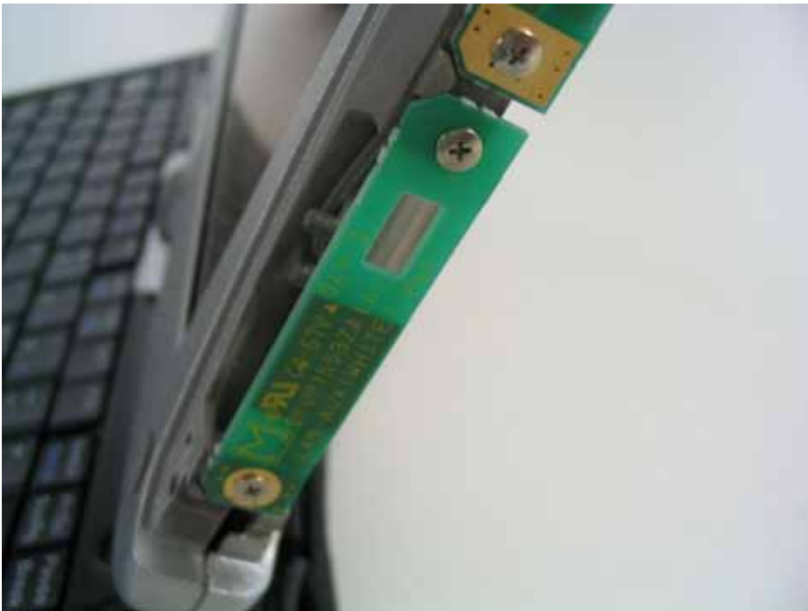
WLAN AUX TX/RX Antenna
