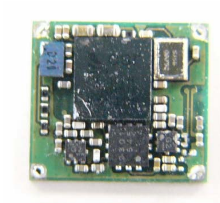
BlueTooth Module inside Top View
