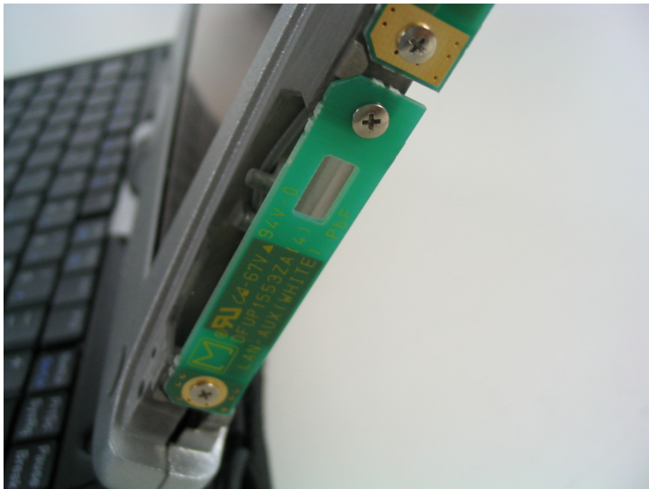
WLAN AUX TX/RX Antenna
