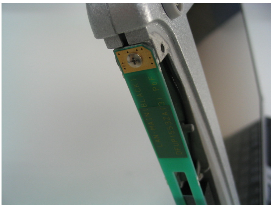
WLAN Main TX/RX Antenna
