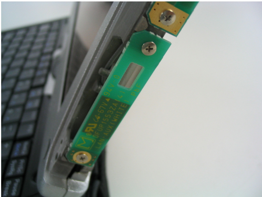
WLAN AUX TX/RX Antenna
