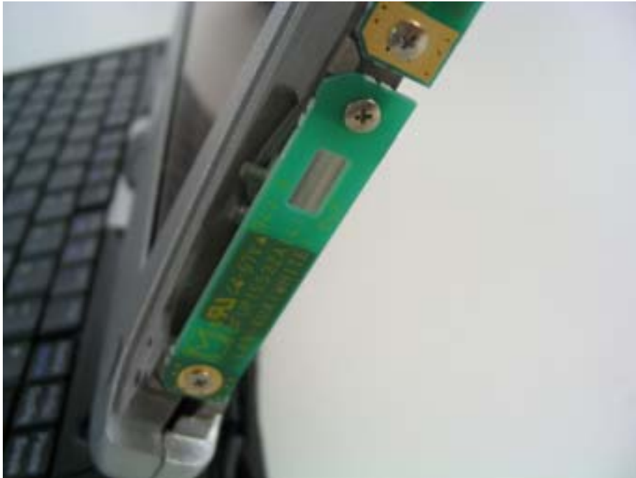
WLAN AUX TX/RX Antenna
