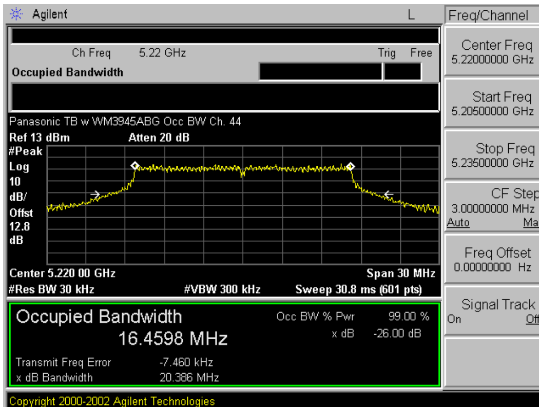
Plot 6-2. 26dB Bandwidth Plot (802.11a (UNII) – Ch. 44)
