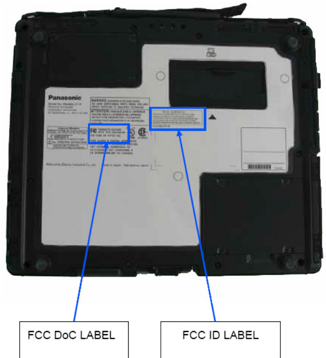
Figure A-3. FCC ID Label Location
