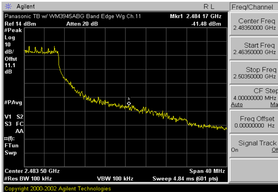
Plot 6-22. Band Edge Plot (802.11g – Ch. 11)
