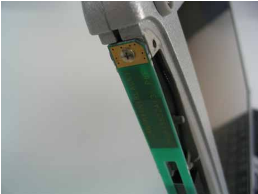
WLAN Main TX/RX Antenna
