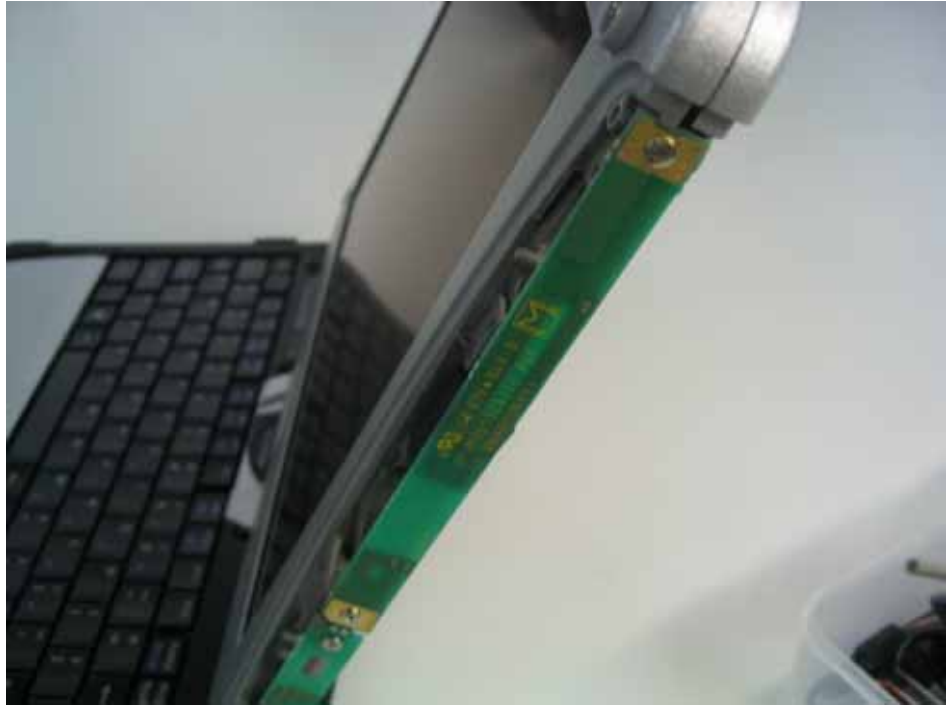
EVDO Main TX/RX Antenna
