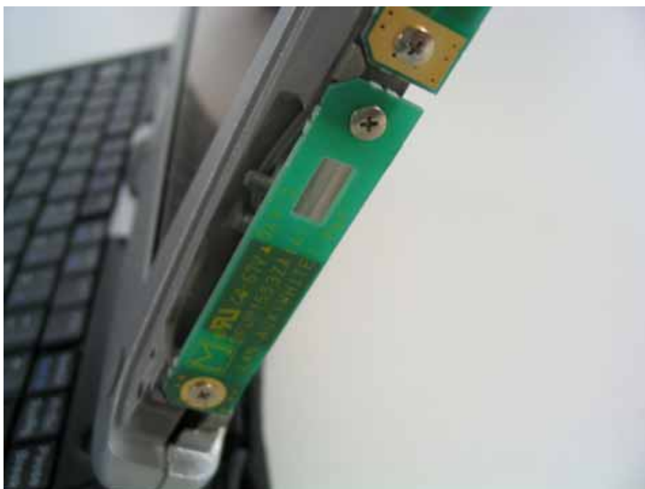
WLAN AUX TX/RX Antenna
