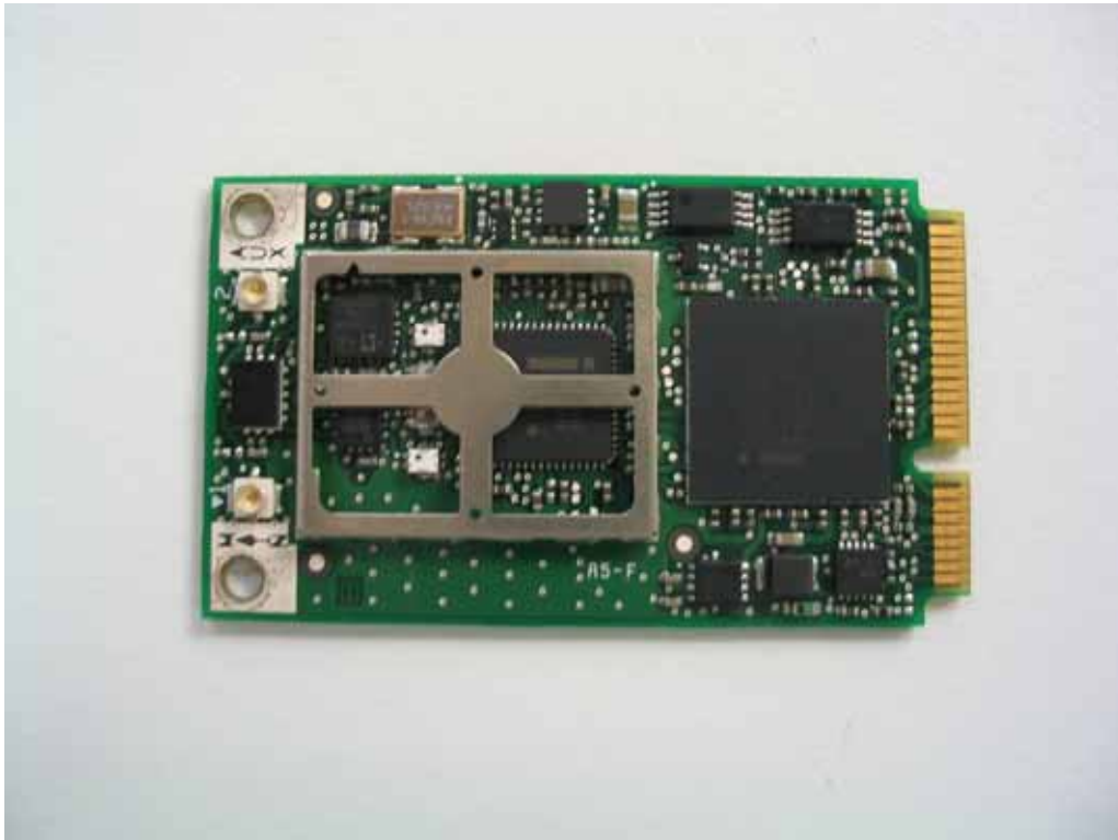
WLAN inside Top View
