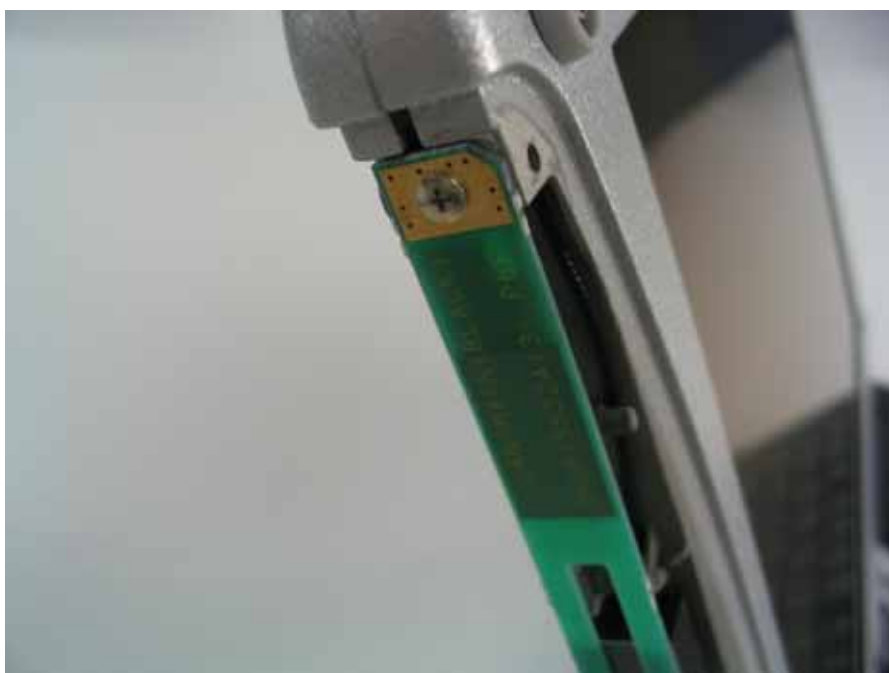
WLAN Main TX/RX Antenna
