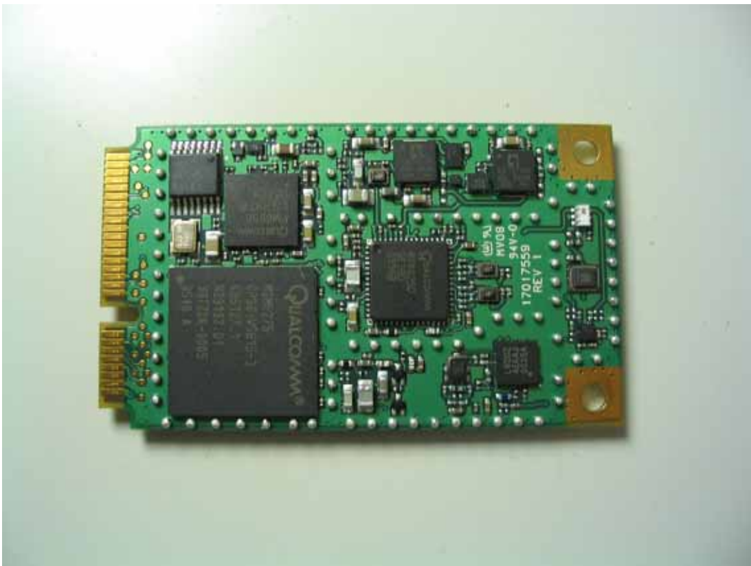
HSDPA Module Interior Bottom View
