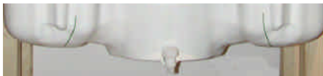
Figure 7.2 SAM Twin Phantom shell
