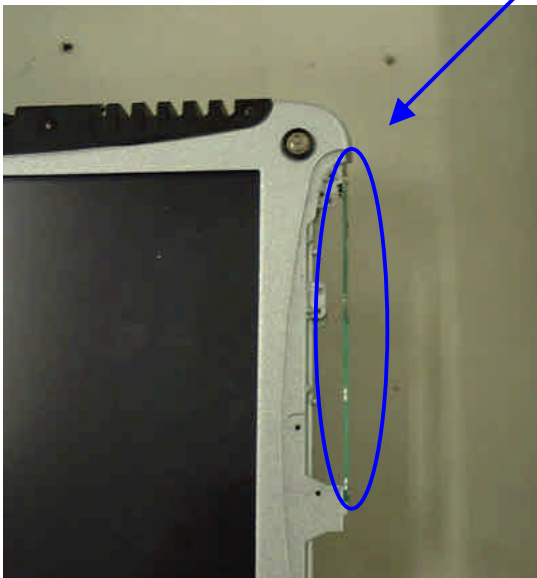
Antenna cover open view
