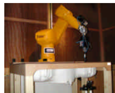
Figure 6.1 DASY4 Test System
