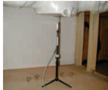
Figure 12.1 Dipole Validation Test Setup
