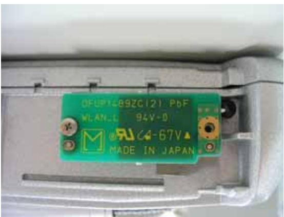
WLAN Antenna View
