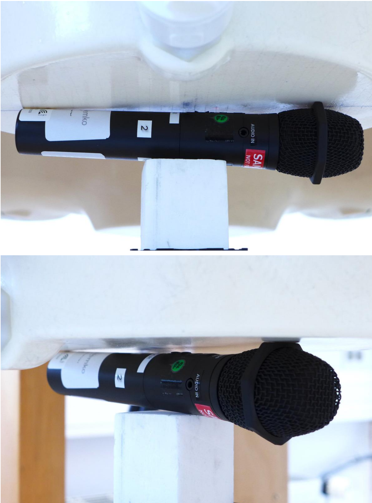
Pic. 3: Test position 1, DUT towards the phantom, 0 mm gap.
