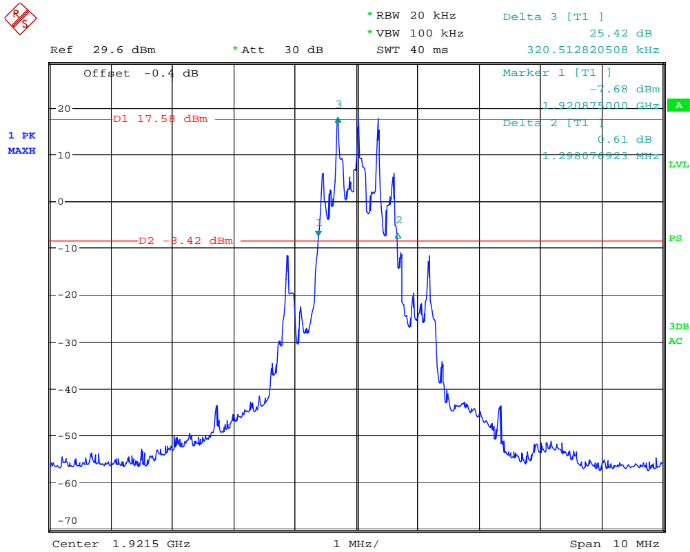
Figure 5: 26dB Bandwidth of 1921.536MHz
