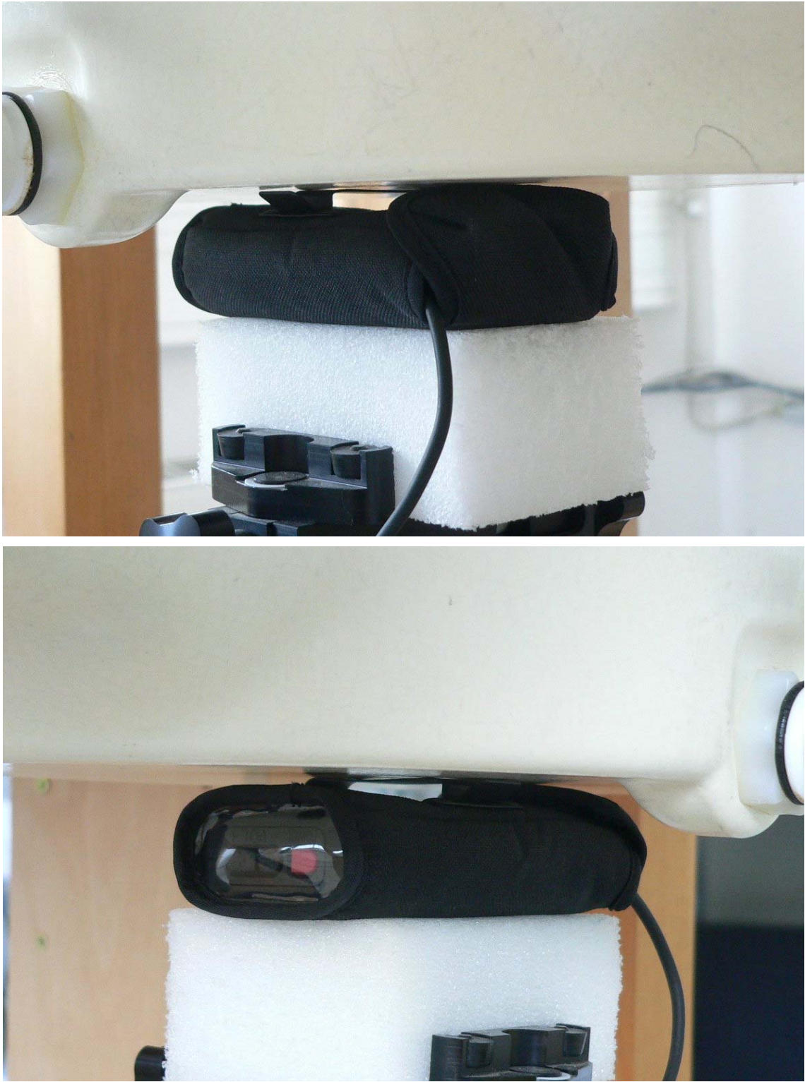
Fig. 12: Body worn configuration for WX-CT420 with attached headset and belt case, position 3, 0 mm distance.
