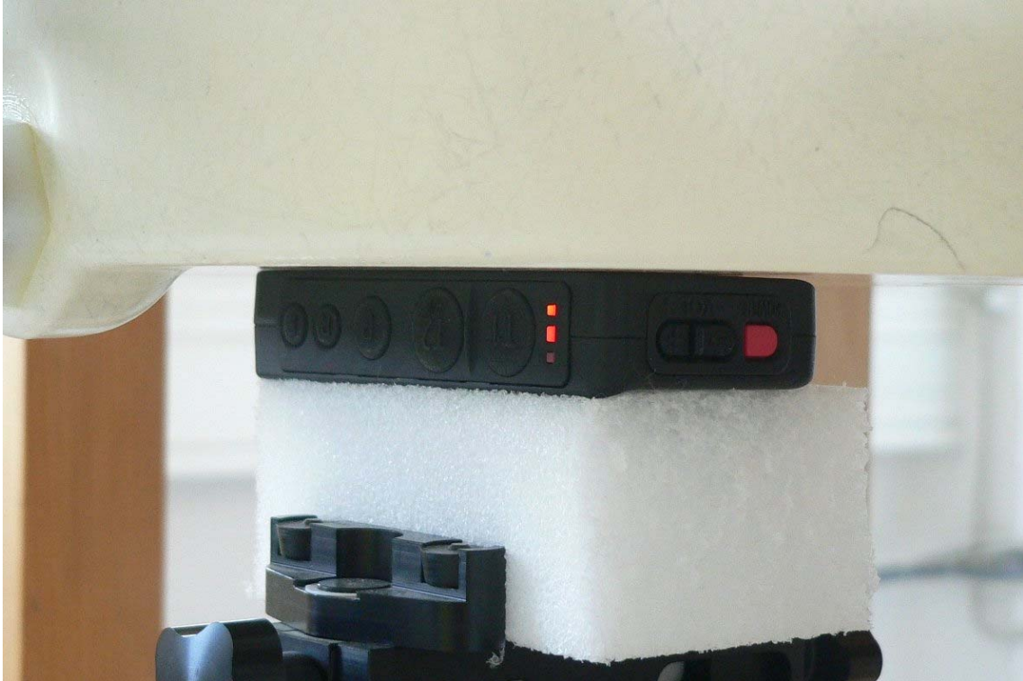
Fig. 10: Body worn configuration for WX-CT420 with attached headset, position 1, 0 mm distance.
