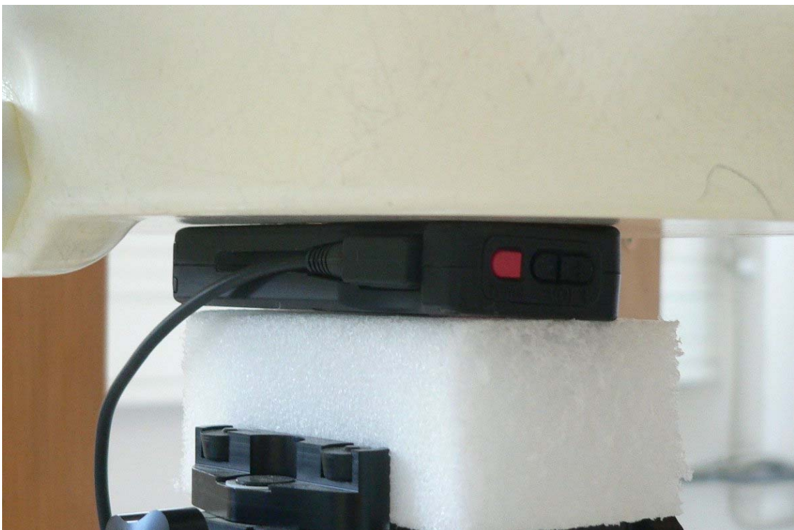
Fig. 11: Body worn configuration for WX-CT420 with attached headset, position 2, 0 mm distance.
