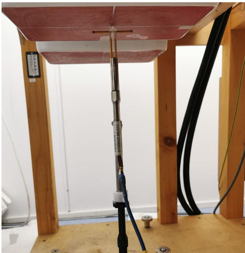
Figure 3 System setup. In system check the DUT is replaced by a verification dipole
