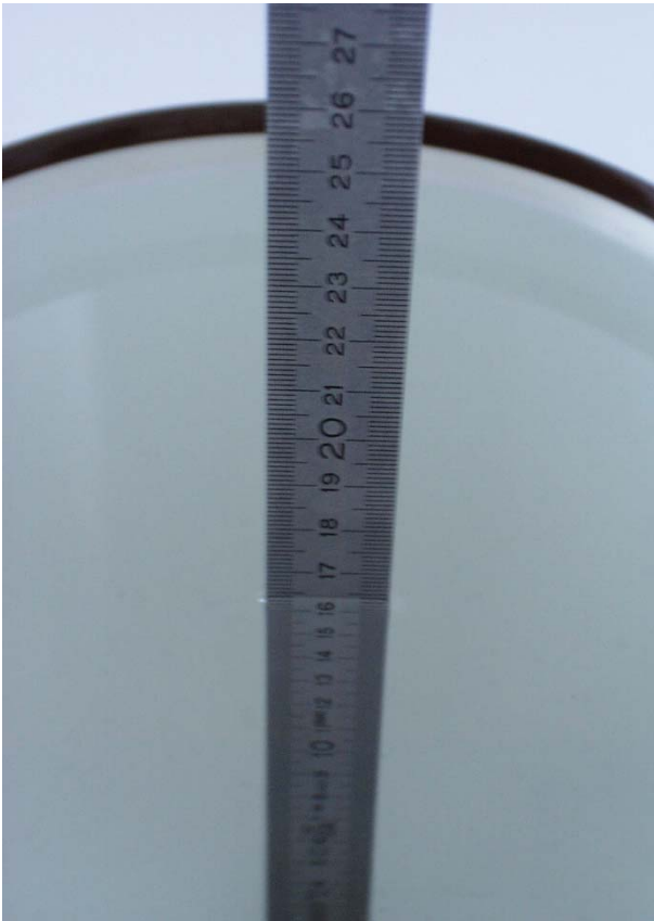
Fig. 17: Liquid depth for 1900 MHz Head measurements
