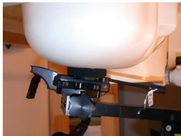
Figure 14.1 Right Head SAR Test Setup -- Check / Touch Position --
