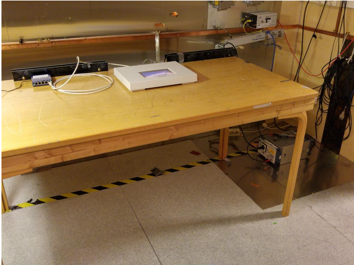
Power line Conducted Emissions Test
