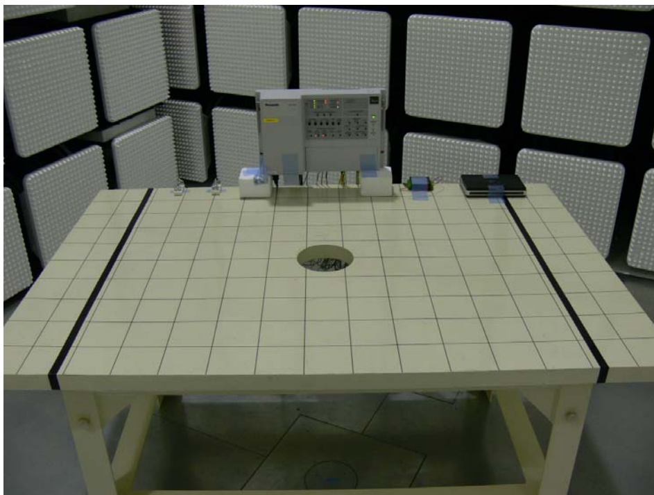
Photograph 3: Set-up for Radiated Emission, EUT Configuration, Front View
