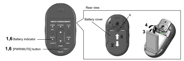
1 Turn off the power by pressing the [PWR/MUTE] button for 2 seconds or more. Confirm that the battery indicator is off.
