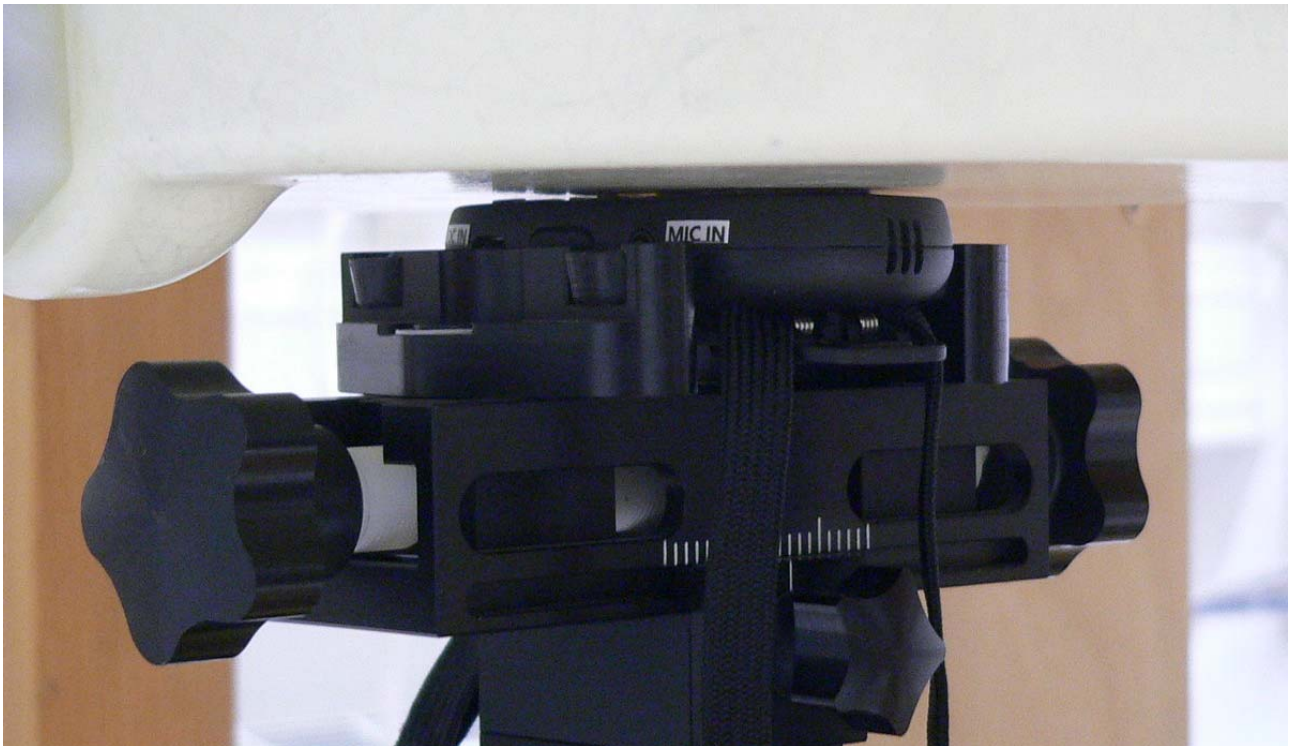
Fig. 9: Body worn configuration for K-STD14, front of the device towards the phantom, belt clip attached, 0 mm distance.
