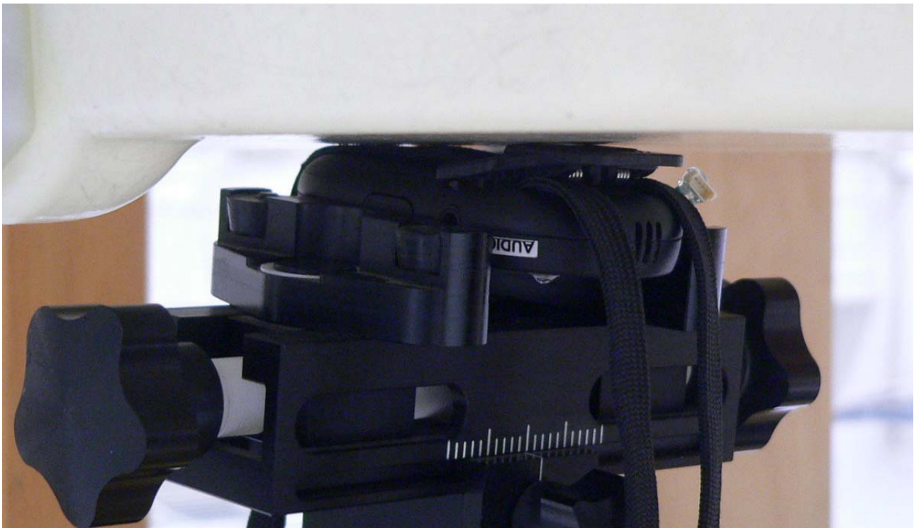
Fig. 10: Body worn configuration for K-STD14, back of the device towards the phantom, belt clip attached, 0 mm distance.
