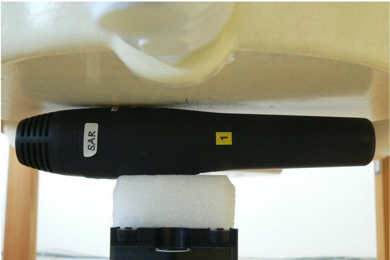
Fig. 13: Test position 4, right side of the K-SHH14 towards the flat part of SAM phantom, 0 mm distance.
