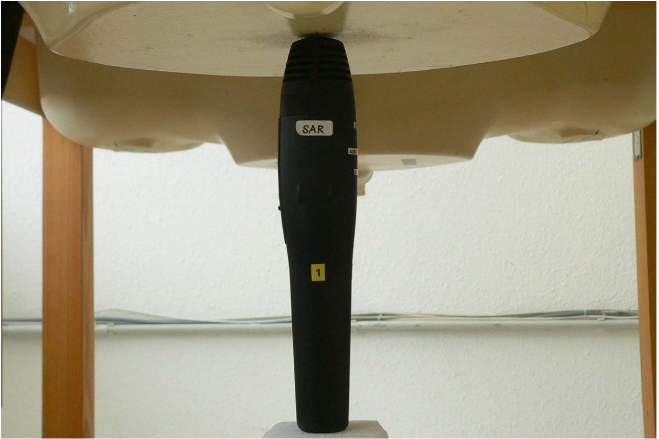
Fig. 14: Test position 5, top side of the K-SHH14 towards the flat part of SAM phantom, 0 mm distance.
