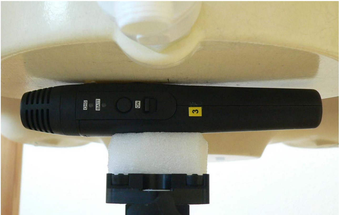
Fig. 10: Test position 1, front of the K-SHH14 towards the flat part of SAM phantom, 0 mm distance.
