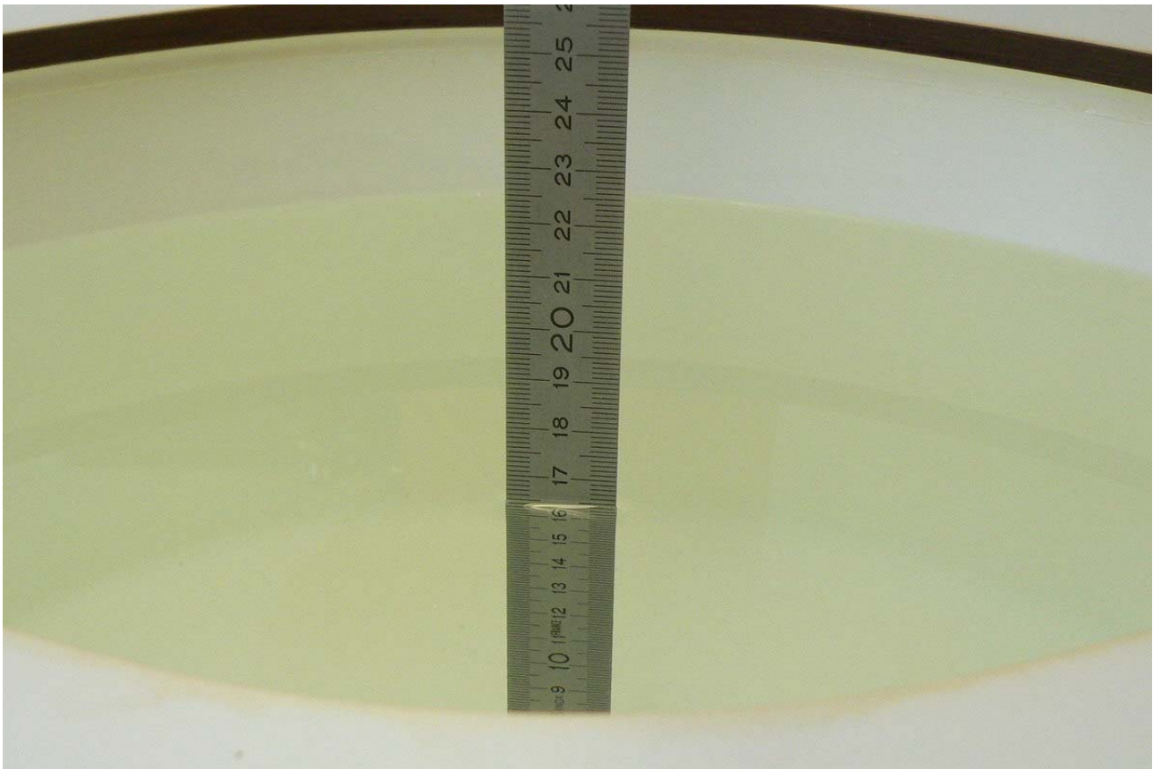
Fig. 15: Liquid depth for 1900 MHz head tissue simulating.
