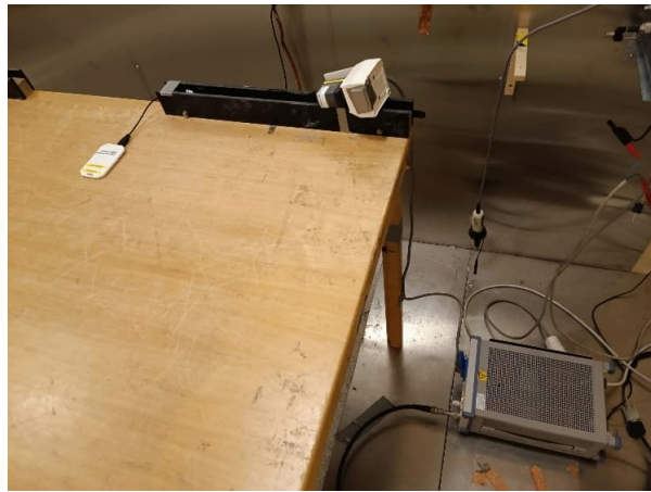
Power-Line Conducted Emissions
