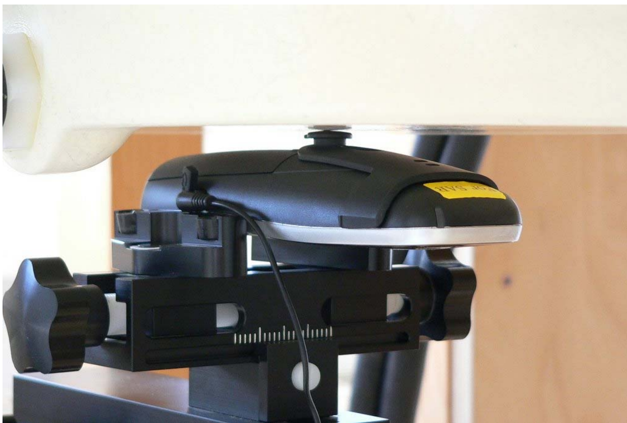
Fig. 21: Body worn configuration , with headset attached, display towards the ground.
