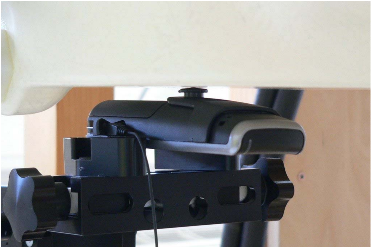
Fig. 9: Body worn configuration for KX-UDT111, position 2, display towards the ground, headset attached, 0 mm distance.
