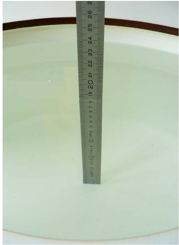
Fig. 23: Liquid depth for 1900 MHz Body worn measurements
