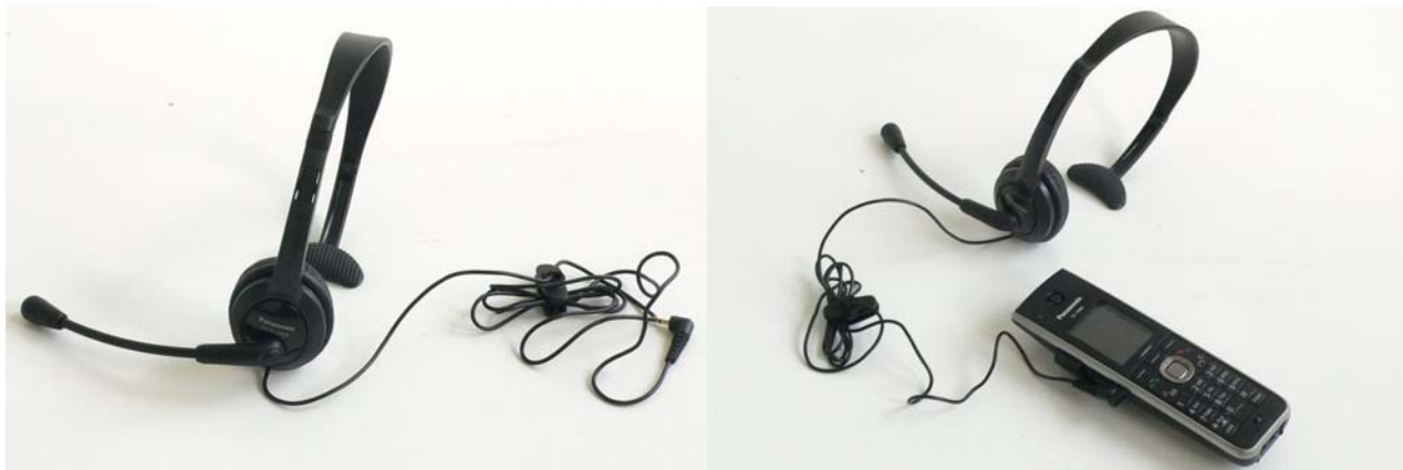
Fig. 13: Pictures of the used headset KX-TCA430.
