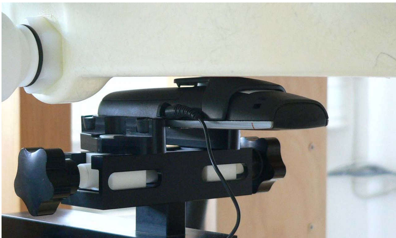
Fig. 19: Body worn configuration for KX-TPA60, back of the device towards the phantom, headset and belt clip attached, 0 mm distance.
