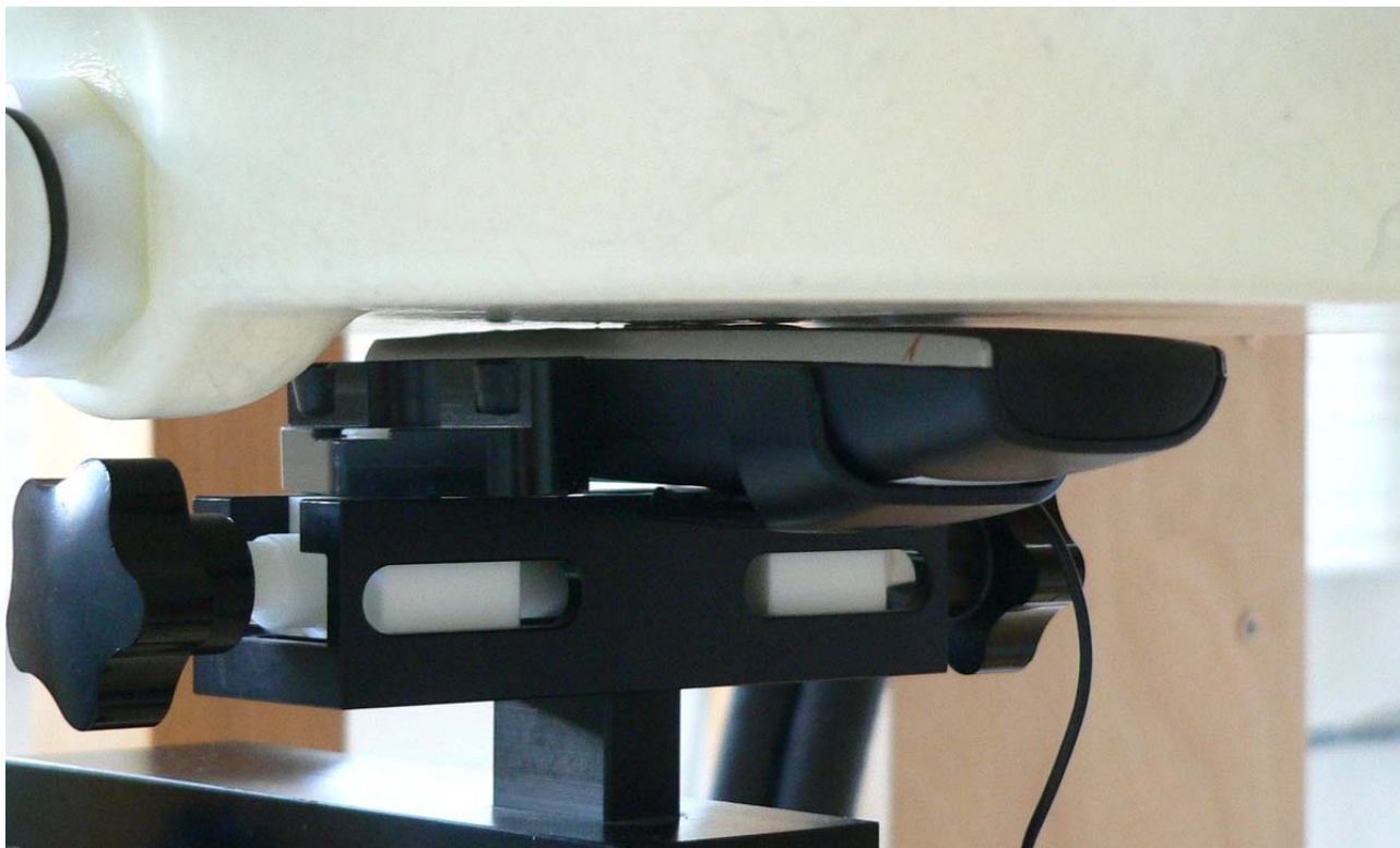
Fig. 18: Body worn configuration for KX-TPA60, front of the device towards the phantom, headset and belt clip attached, 0 mm distance.
