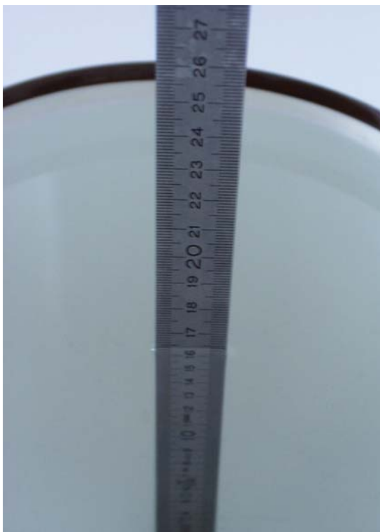
Fig. 20: Liquid depth for 1900 MHz Head measurements
