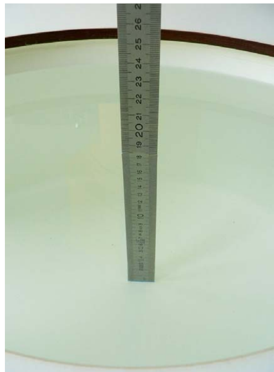
Fig. 21: Liquid depth for 1900 Body worn measurements
