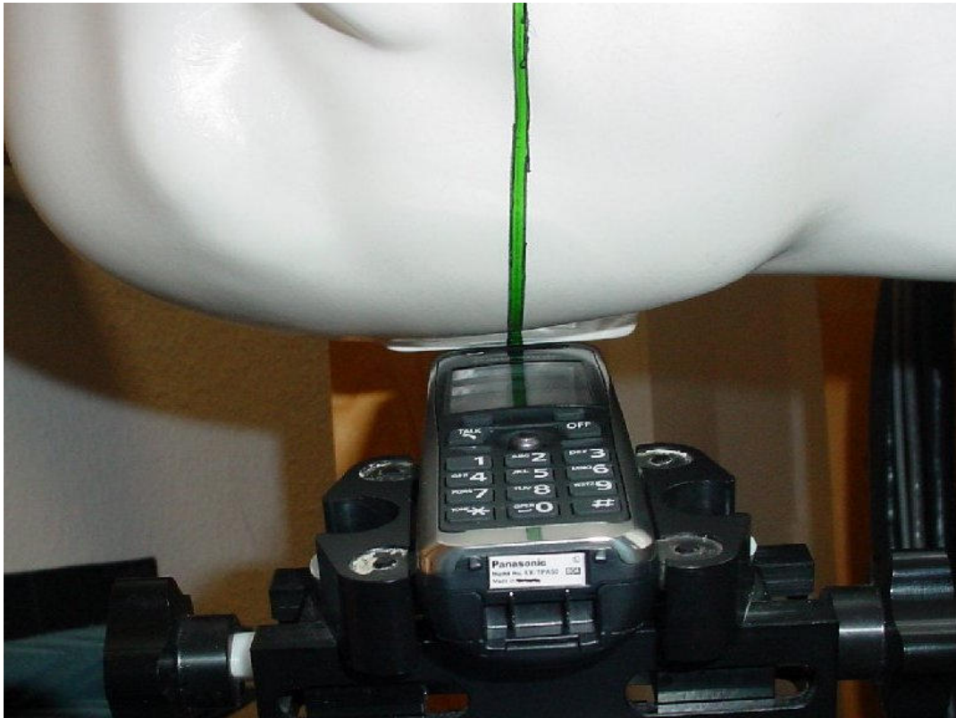
Photo 16: Test position right hand tilted 15°
