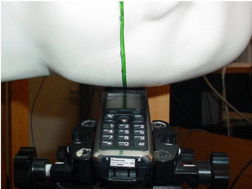
Photo 10: Test position left hand tilted 15°
