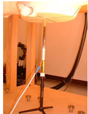
2450MHz System performance check setup
