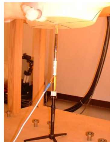
2450MHz System performance check setup
