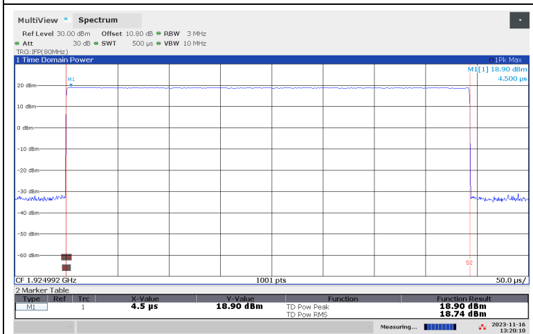
Conducted Peak Output Power, Middle Channel
