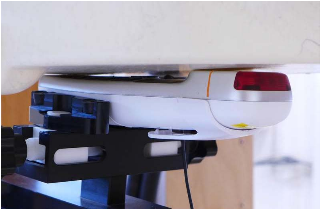
Fig. 19: Body worn configuration for KX-TGMA45, front of the device towards the phantom, headset attached, 0 mm distance.
