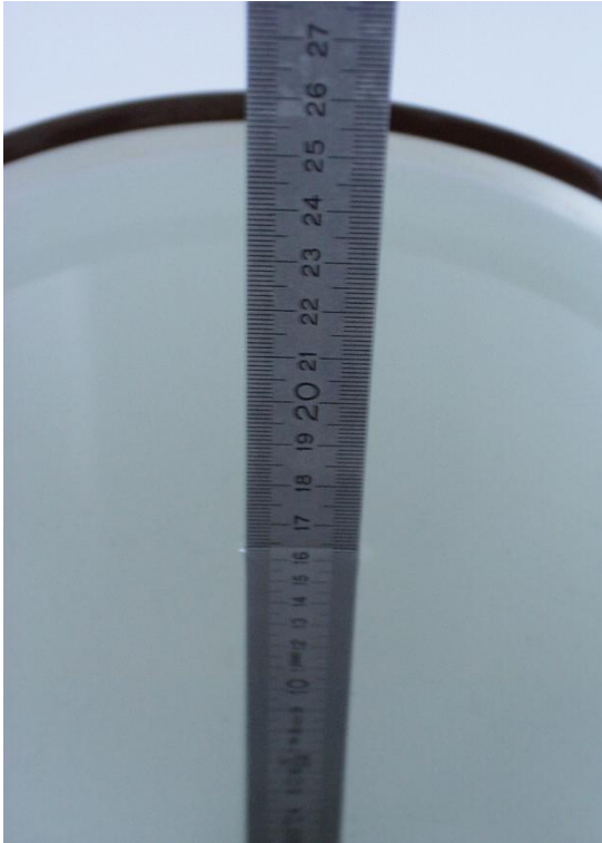
Fig. 17: Liquid depth for 1900 MHz Head measurements
