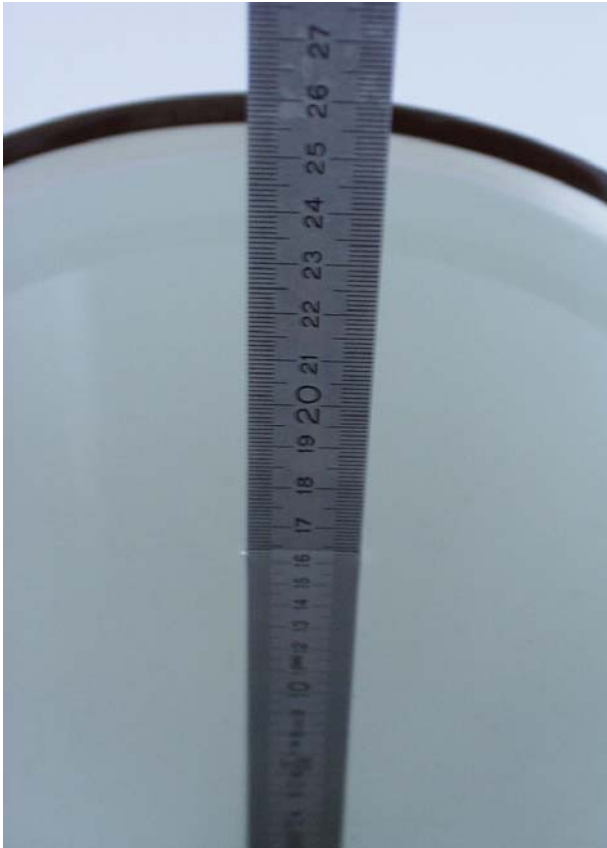
Fig. 17: Liquid depth for 1900 MHz Head measurements
